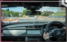
The stereo camera uses advanced image processing software to recognise roadworks and can guide the vehicle to the centre of the lane, even when road markings are faint or missing.
