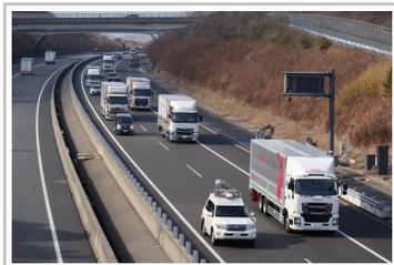
Daimler testet Truck Platooning in Japan.
